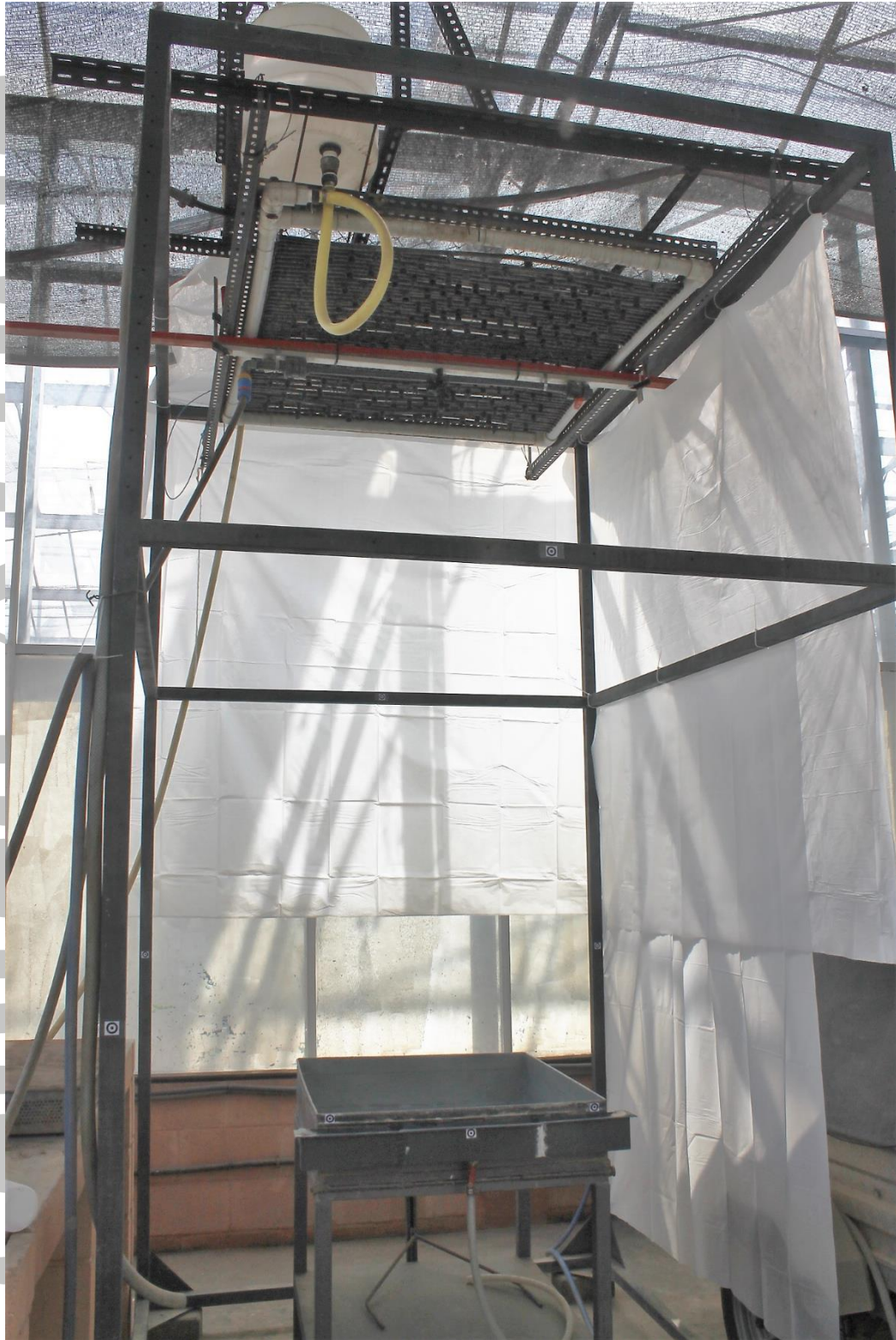
Figure 2 Rainfall simulator used in the experiment, showing the supporting structure, the soil box (bottom) and the droplet generator array (top). Note the distribution of GCPs at different heights and depths on the structure and soil box. The transparent plastic hose in the front of the box was used to collect runoff. There is another hose to collect infiltration which is not visible in the picture.
