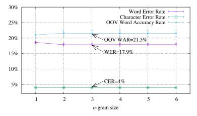
**Figure 17.** Results obtained by the CRNN word-based system using *n*-gram language models with size  $n = \{1, ..., 6\}$ .
