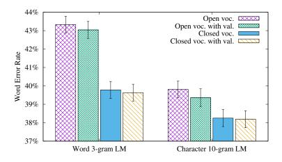
**Figure 13.** WER results obtained by the best word-based HMM system and the best character-based HMM system with open and closed vocabulary, with and without using the validation samples for training the LM.
