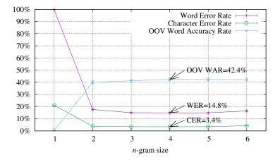
**Figure 18.** Results obtained by the CRNN sub-word-based system using *n*-gram language models with size  $n = \{1, ..., 6\}$ .
