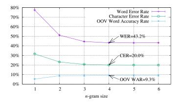
**Figure 8.** Results obtained by decoding at the HMM sub-word level by using *n*-gram language models with size  $n = \{1, ..., 6\}$ .
