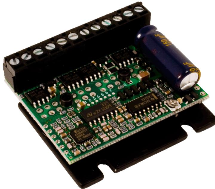
Figura 59: Controladora GeckoDrive G251X
