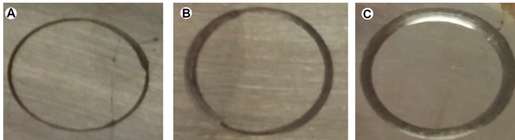
Figure 3. Wear tracks for (A) group 1, (B) group 2 (preheated at 450 °C) and (C) group 3 samples (annealed at 900 °C).
