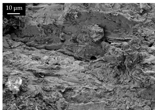
Figure 7. SEM image of the broken surface for group 1 samples.
