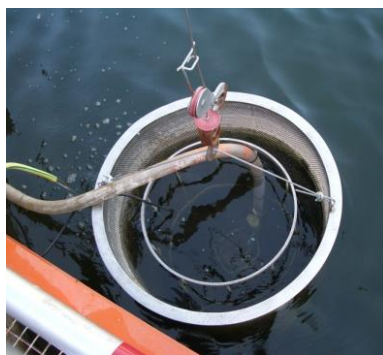
Figure 5. Catchment point with double filter in the Náquera Research Centre (CIN)
