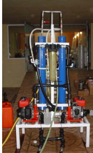
Figure 1. UF plant set up in Pucará (Ecuador)
