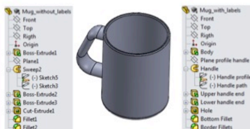
Figure 3. Proper labeling of modeling operations as a simple way to convey design intent. Default naming (right tree) vs. proper naming (left tree).
