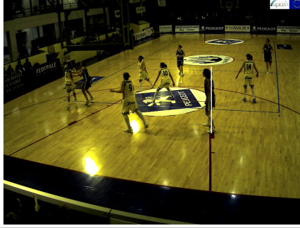
Figure 4.1 An example of a region R_{\mathbf{x}}^n with H = 2m is marked with a white line on the player of the dark team at the front right in the image. The 3D box with as ground plane the cell \mathbf{x} ( \mathbf{x} has an area of (0.02m)^2 ) is so thin, that it is reprojected onto a line-shaped region R_{\mathbf{x}}^n .
