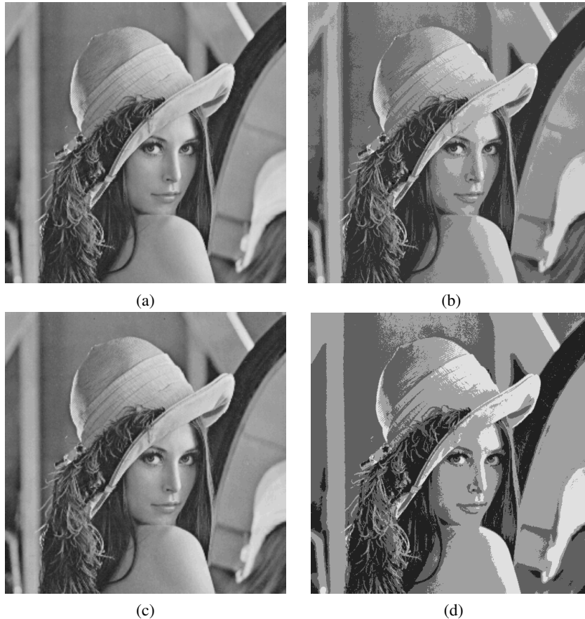
Figure 2.10 Coding of the image Lena using: (a) MPCM-MAP ( s = 32 ) at 3 bpp, (b) PCM at 3 bpp, (c) MPCM-MAP ( s = 32 ) at 2 bpp, and (d) PCM at 2 bpp.
