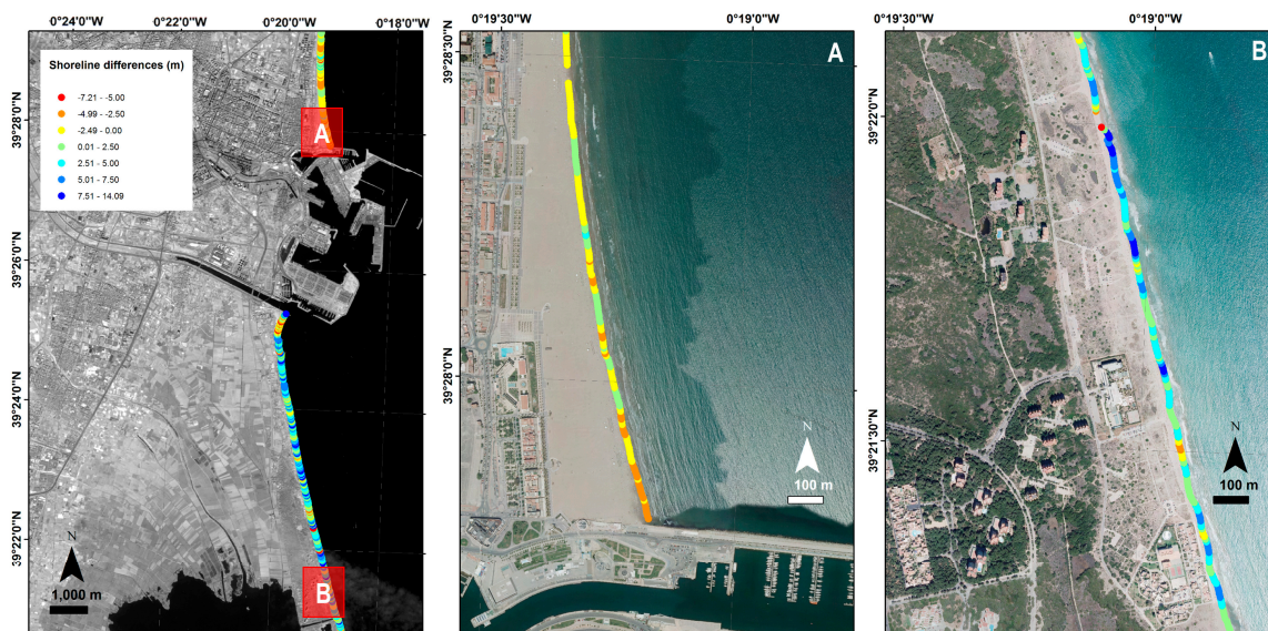
Figure 8. Map shows differences between shorelines for Landsat 8 and Sentinel-2 with a few minutes of difference. Negative values indicate that Landsat 8 is displaced landwards with respect to Sentinel-2, while positive values imply seaward bias. Details (A,B) show the influence of the width of the beach in the shoreline positions due to the differing spatial resolutions of these two types of images.
