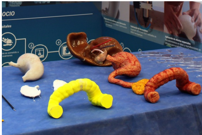
Figure 1. Simula Project. Organs made from 3D printing of models and molds, reproductions with silicones. Degree work. Student: I.D. Leonel Hernández. Director: Prof: Juan Avila El Bosque University. 2016
