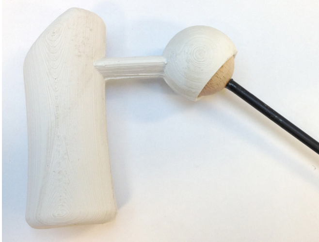
Figure 67. PF prototype used during the MoCap experiment. The handle has a cylindrical shape in order to avoid the pain caused by the rings of the conventional pistol-grip handle.
