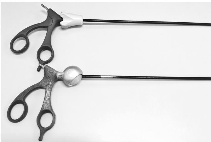
Figure 39. Both instrument used to compare the effectiveness of PF in hand-held instruments. Superior instrument is a conventional pistol-grip handle. Inferior instrument is the PF prototype.
