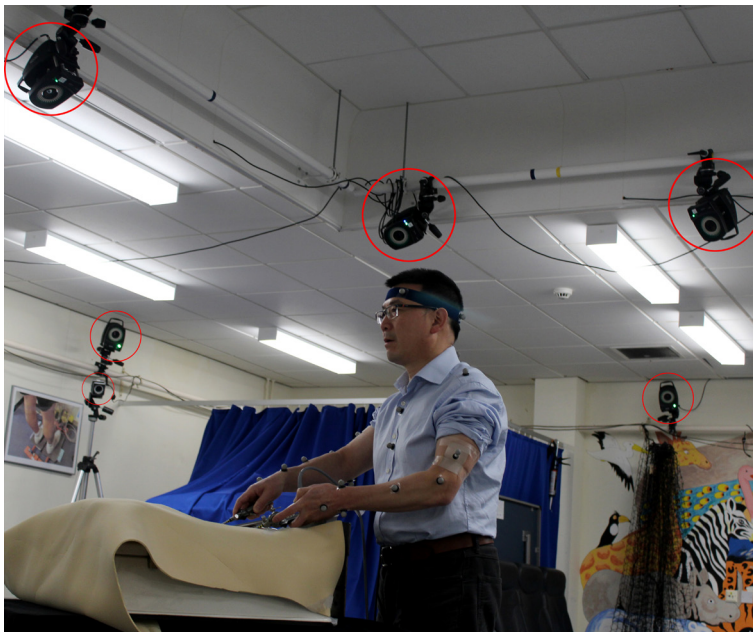
Figure 61. Laparoscopic surgeon being recorded by VICON system. Picture of the study performed at IMSaT laboratory in the Ninewells Hospital (Dundee, Scotland). Red circles mark only a fraction of the cameras used during this experiment.
