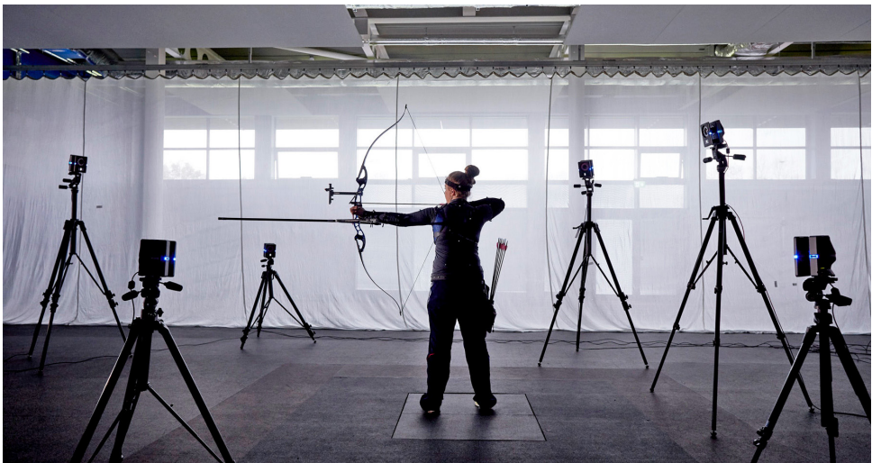
Figure 54. Basic VICON setup to evaluate an archer motions. Acquired from Engadget magazine.
