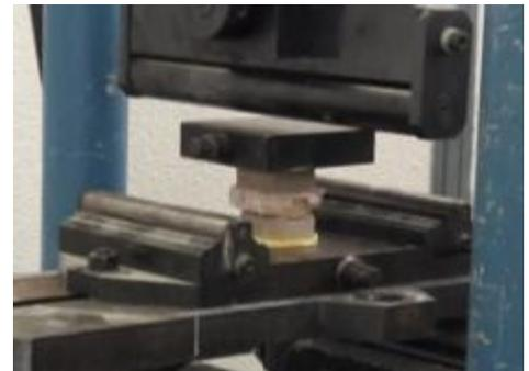
*b- test body positioned in the press*
