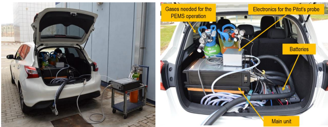
Figure 1. Test vehicle with the portable emissions measurement system installed. The calibration equipment is shown in the left-hand side picture.
