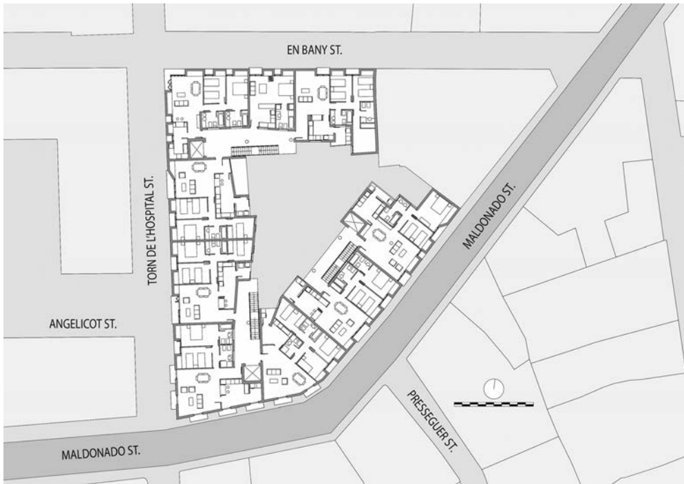
Figure 3. Maldonado building. First-floor layout, which shows the contrast between the external shell of a ninety-centimeter-thick façade that allows the built-in furniture, balconies, and the broken and open internal façade to be created. (Image by Fernando Vegas and Camilla Mileto, 2017)
