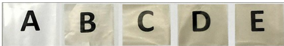
Fig. 2. Photographs of films containing: (A) neat EVOH 10%; (B) EVOH/CNC (0.3% wt.-%)/ PdNP (0.3 wt.-%); (C) EVOH/CNC (0.6 wt.-%)/PdNP (0.6 wt.-%); (D) EVOH/CNC (1 wt.-%)/PdNP (1 wt.-%); (E) EVOH/TOCNC (1 wt.-%)/PdNP (1 wt.-%).
