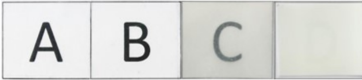
Figure 6. Contact transparency of the poly(3-hydroxybutyrate) (PHB) films prepared at various annealing times for up to 5 min and cooled in air at room temperature: (A) t_0 ; (B) t_5 ; (C). Compression molded PHB film; (D) Electrospun PHB fibers without heat treatment (opaque material, D letter underneath not discernible).
