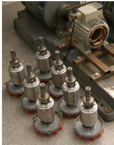
Figure 9. Tested rotors with two broken bars in different relative positions, with the stator used for performing all the experimental tests.
