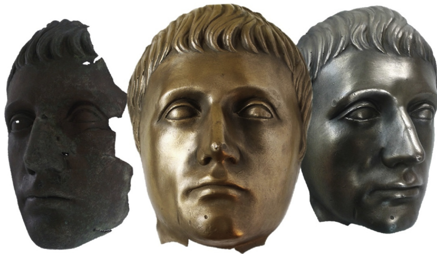
Fig. 1. Different finishes of metal composites produced in this study based on vinyl ester resin for heritage cloning, by using a mould of a roman Augustus head. From left to right a patinated bronze; a burnished bronze and burnished iron.
