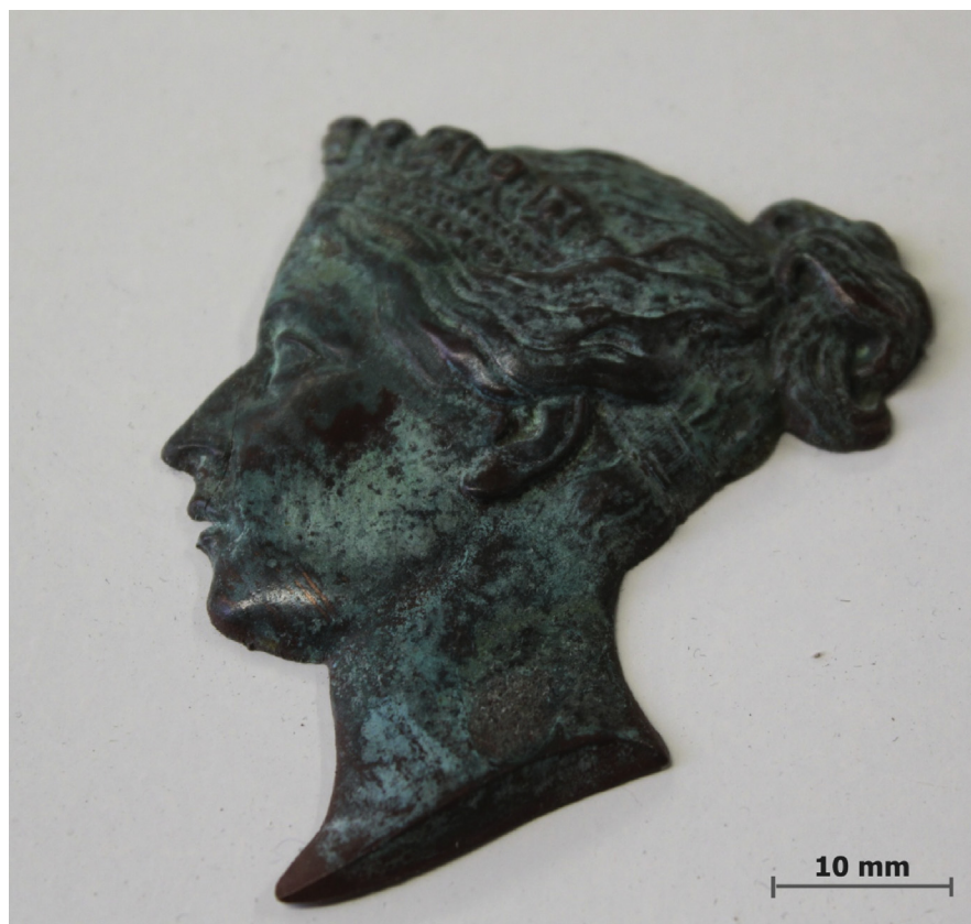
Fig. 3. An artificial copper 80% wt based on epoxy resin used in this study as a decorative figurine. The vat patina has been developed with ammonia in a 48 hours cycle.
