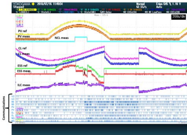
Fig. 14. Set of IoE communications (down), control signals and flows of Energy (up) in the application example under consideration
