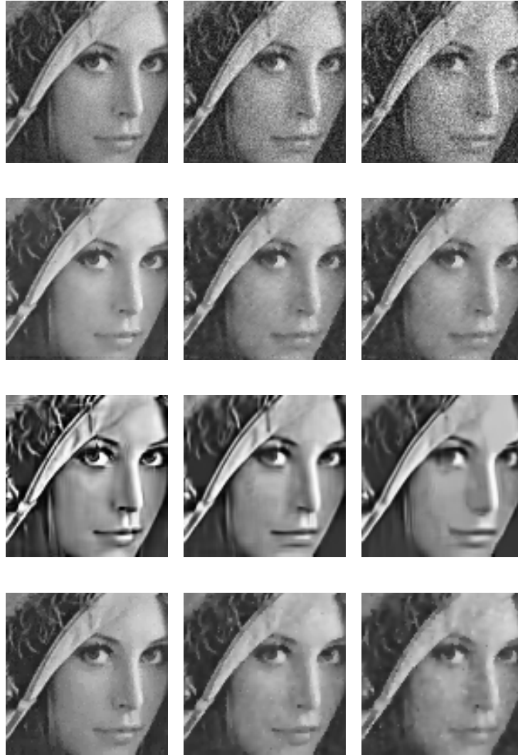
Fig. 1.12: First row, Lenna image corrupted by Gaussian noise with standard deviations \sigma = 10 , \sigma = 20 and \sigma = 30 . Second row, the output of Fuzzy Network filter. Third row, output of BM3DShar and in the last one, the output of TeD-FAB.
