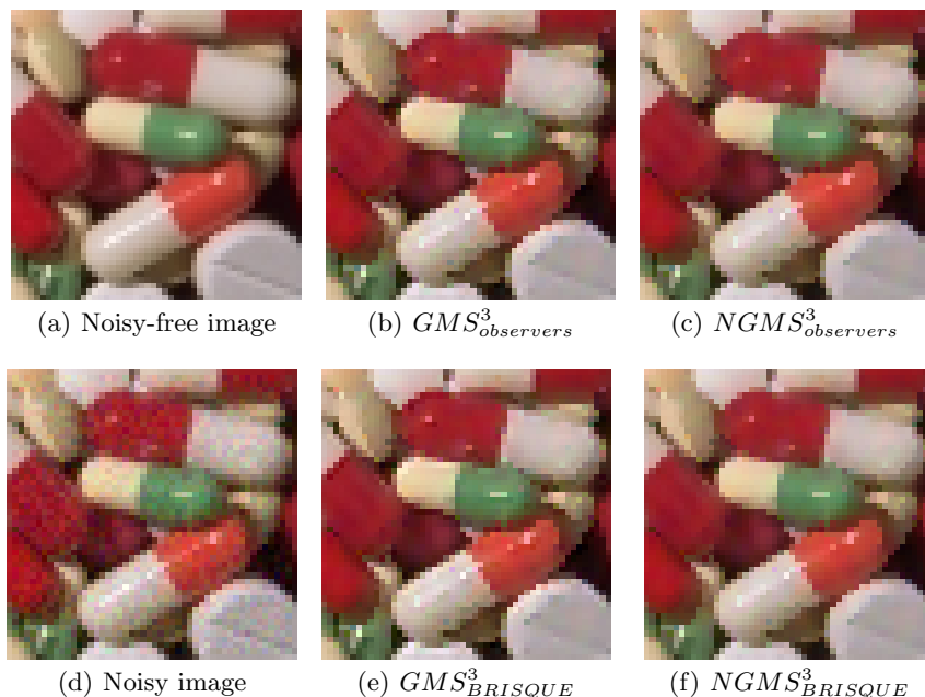
Fig. 6.16: Examples of filtering with GMS^3 and NGMS^3 using the parameters set by observers (b) & (c) and with the optimal parameters fixed by using BRISQUE score (e) & (f).
