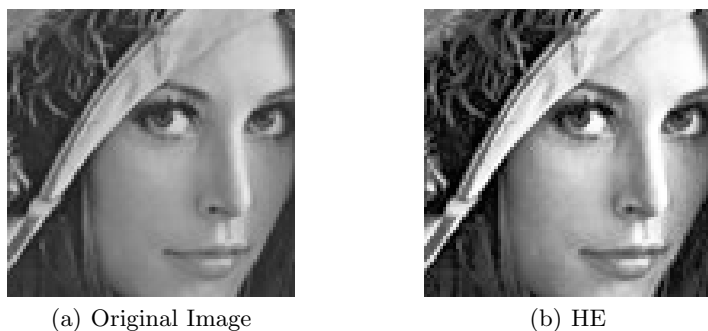
Fig. 1.4: Comparison between a gray-scale image of Lenna and the resulting image after having applied HE.
