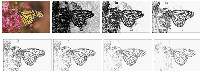
Fig. 4.11: Evolution of the border detection in function of the threshold, from \mathcal{U} = 5 to \mathcal{U} = 70
