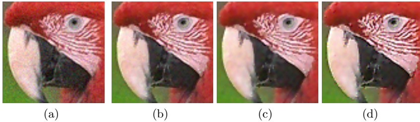
Fig. 6.7: Examples of application of GMS^3 method. From left to right: (a) original noisy image with \sigma = 5 , (b) processed image with \alpha = 3 , \lambda = 0.2 , (c) processed image with \alpha = 5 , \lambda = 0.2 , and (d) processed image with \alpha = 5 , \lambda = 0.8 .
