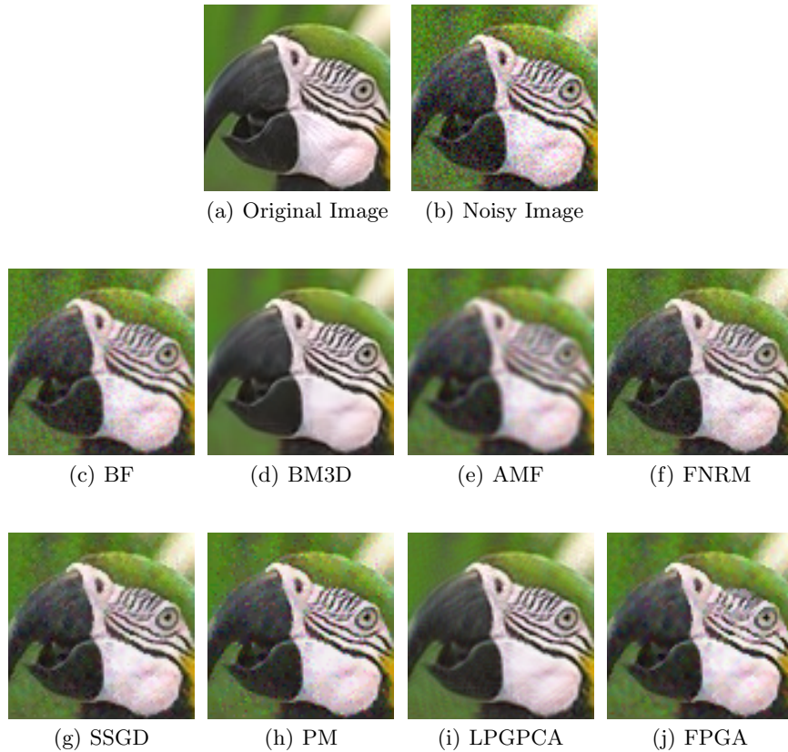
Fig. 1.2: Results under different smoothing methods applied to Parrots image corrupted by a Gaussian noise with standard deviation \sigma = 20 .
