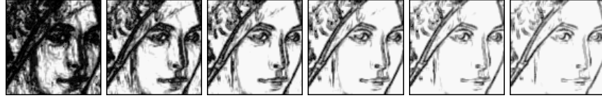
Fig. 4.10: Evolution of the border detection in function of the threshold of the Lenna image, from \mathcal{U} = 10 to \mathcal{U} = 60
