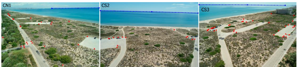
Fig. 2.5. Three examples of photos at El Saler beach taken from different camera position on 17 June 2016; the first photo from the north camera (NC) and the other two from the south camera (CS). Distribution of the GPS points in the area is dotted in red and the horizon line is shown in blue. CN1 is an example of where the horizon formulas are obtained by two points, while CS2 and CS3 are obtained by three points.
