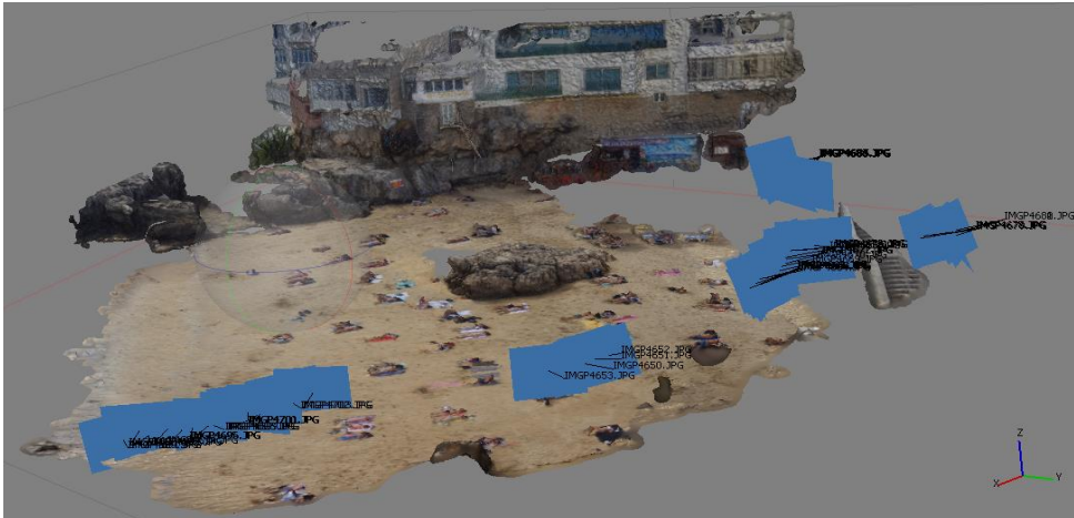
Fig. 5.37. Dense point cloud and 3D reconstruction of Praia da Rainha. The blue rectangles represent the cameras taken by sets of photos from different positions.
