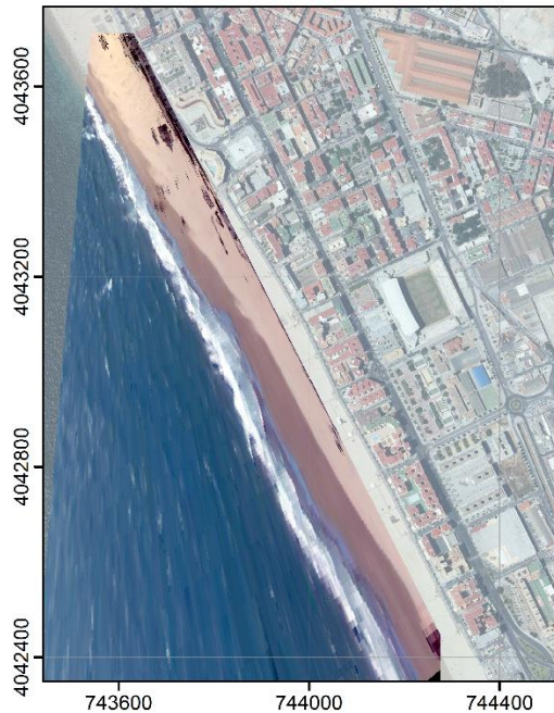
Fig. 6.2. C-Pro projection map with an instantaneous photo of the southern camera of Horus system for 31/03/2016 at ebbing tide in Victoria beach (Cádiz, Spain). Grid coordinates: GCS_ETRS89 UTM29N.
