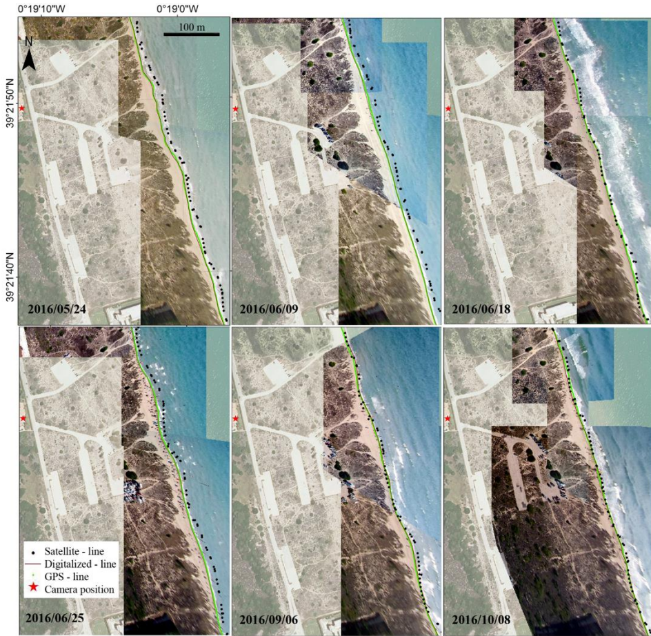
Fig. 4.18. The same 2010 PNOA orthophoto is used in the six maps simply as a basemap. Above it, the projection of the terrestrial photos of six different days for El Saler beach is shown. Their projection is made at the mean sea level value for each date. Note that the camera is not fixed, and the different extension covered by the photos is a consequence of the hand-selected region projected. Each map shows the GPS-line, the digitalised-line (almost coincident between them) and the satellite shoreline.
