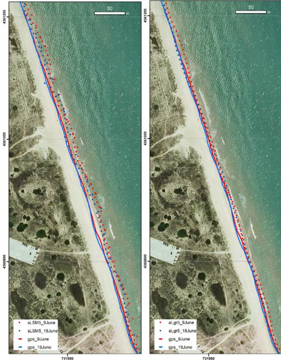
Fig. 3.11. Coastal segment of El Saler beach where different shoreline solutions are shown for 9 and 18 June in red and blue respectively. The GPS shorelines are represented with lines and the sub-pixel shoreline solutions with dots (sLSM5 and the
