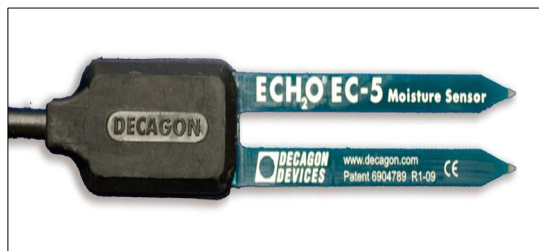
Figura 12. Sensor FDR (EC – 5, Decagon Dervices Inc., Pullman, WA).
