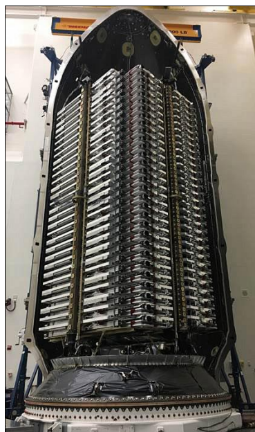
Figure 2. Starlink 60 satellites in Falcon 9's fairing. Ref [18]
