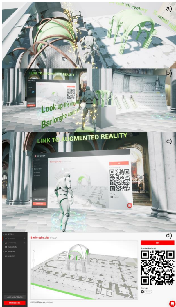
Figure 10: The links between VR and AR by QR codes: a,b,c) allow the creation of an AR CDE; d) able to show a huge quantity of information connected to the model and the reality, supporting further analysis directly in the field.
