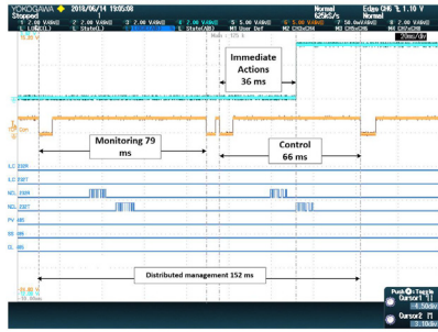
Fig.11. Response times of the exchanged messages by using RR communication
