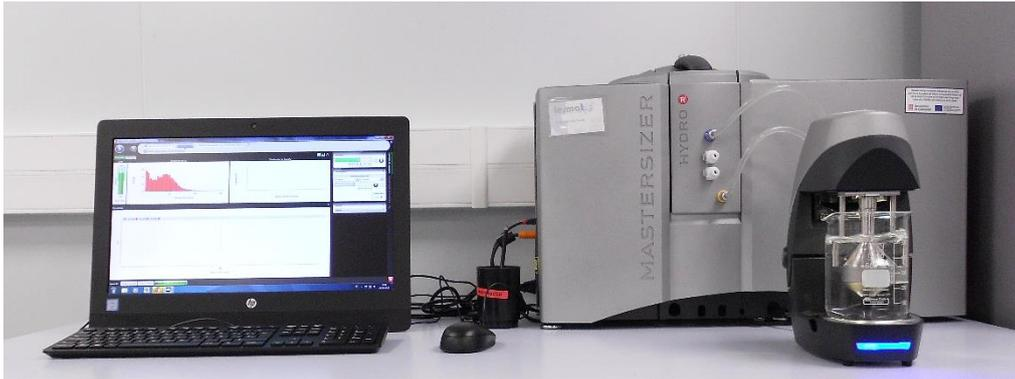
Figure 12. Mastersizer 3000E Hydro EV.
