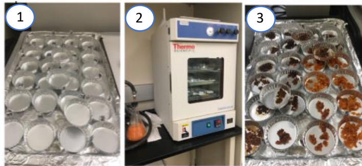
Figure 9. Labeled pans for samples of each time point (1); vacuum oven (2); samples after 22 h at 110°C (3).
