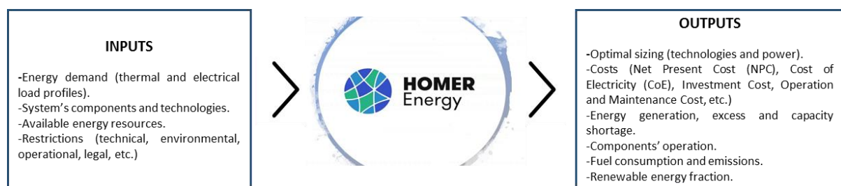
Figure 25. Schematic overview of inputs and outputs of HOMER Software. Source: Own elaboration
