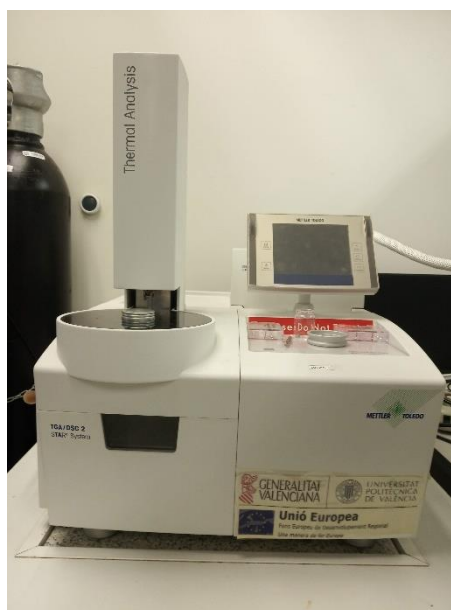
Figure 17. TGA/DSC 1 star system METTLER TOLEDO on which TGA measurements were taken.
