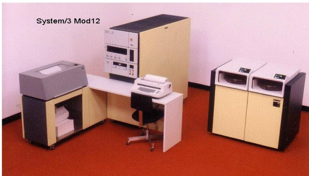
**Figura 2.20:** IBM System/3 Modelo 12
