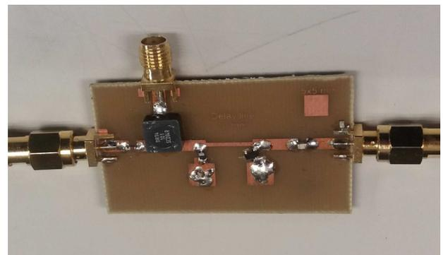
**Figure 4.** The designed system with SRD pulse sharpener and the corresponding equivalent Layout circuit.
