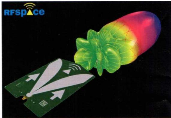
**Figure 6.** Photograph of the UWB antenna with the radiation pattern.
