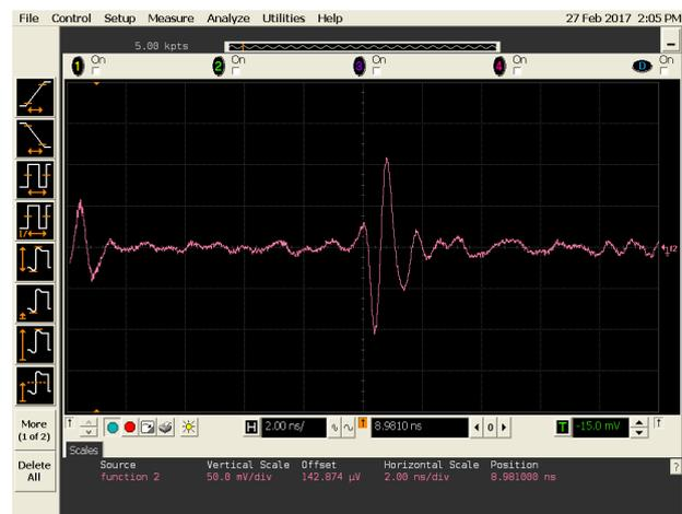
**Figure 8.** The time-domain response of the radar sensor measurement towards a metal plate located at  $50cm$ .
