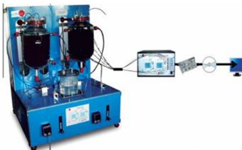
Fig. 1. Picture of the computer controlled anaerobic digester (PDANC model) set-up used for the study (EDIBON, 2014).
