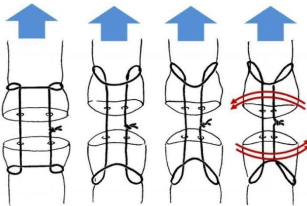
**Fig. 6.-** Phenomenon of axialization and rotation of the tendon near the cut edge
