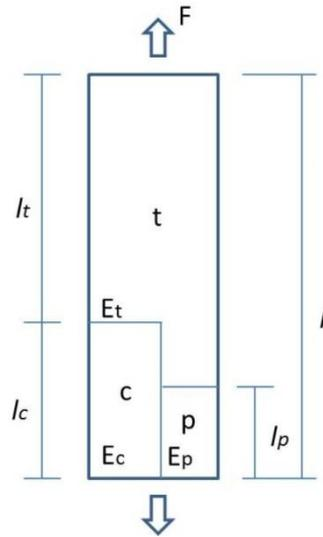
**Fig. 5.-** Model of tendon with core suture plus epitendinous peripheral.
