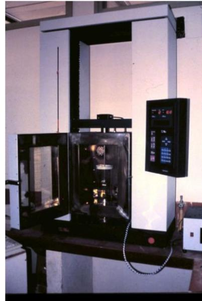
**Fig. 2.-** DY.34 (Adamel Lhomargy S.A.) mechanical testing machine.
