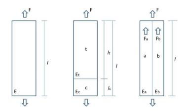
**Fig. 4.-** Mechanical model: a) single element; b) tendon plus core suture associated in series; c) two elements associated in parallel.
