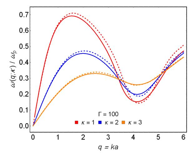
Figure 4.13. Dispersion relation for the YOCP mode. Solid lines represent the exact solution of (4.9), dashed lines represent the exact solution of (4.9), but with moments, calculated from MD DSFs of [32].
