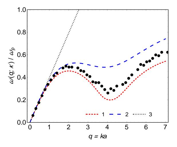
Figure 4.14. Dispersion relation for the YOCP quasiacoustic mode, compared to MD data [32] (dots) at  $\Gamma = 100$  and  $\kappa = 2$ .
