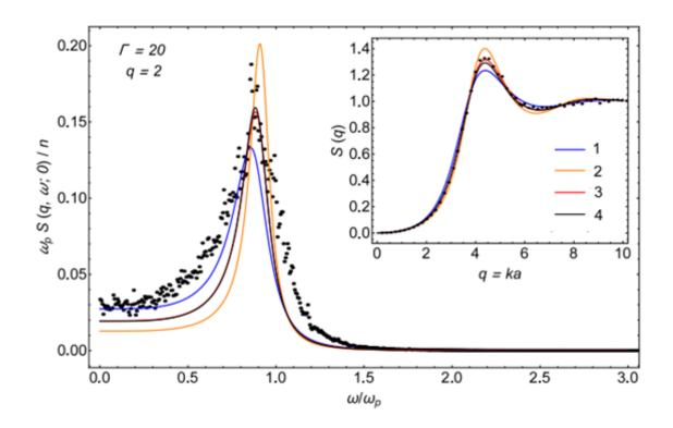
Figure 5.1. Static and dynamic structure factors in COCPs, compared to the MD results (dots) [32]. The static structure factors were calculated using the following schemes: 1 - [30], 2 - [37], 3 - [38,39], 4 - [31].
