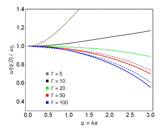
Figure 4.11. Dispersion relation for the COCP mode. Solid lines represent the exact solution of (4.9), dashed lines represent the exact solution of (4.9), but with moments, calculated from MD DSFs of [32].
