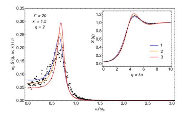
Figure 5.3. Static and dynamic structure factors in YOCP, compared to the MD results (dots) [32]. The static structure factors were calculated using the following schemes: 1 - [30], 2 - [37], 3 - [38,39], 4 - [31].
