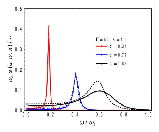
Figure 4.8. The comparison of YOCP DSFs, calculated as eq. (4.7) (lines) and obtained from MD simulations [32] (lines with symbols).
