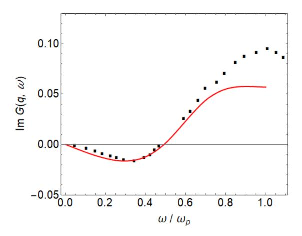
Figure 4.16. Imaginary part of the expression (4.14) for the dynamic local field correction (solid line), compared to the MD results [33] (squares), at q = 1.02 and  $\Gamma = 10$ .
