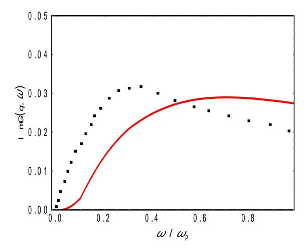
Figure 4.20. Imaginary part of the expression (4.14) for the dynamic local field correction (solid line), compared to the MD results [33] (squares), at q = 1.02 and  $\Gamma = 120$ .
