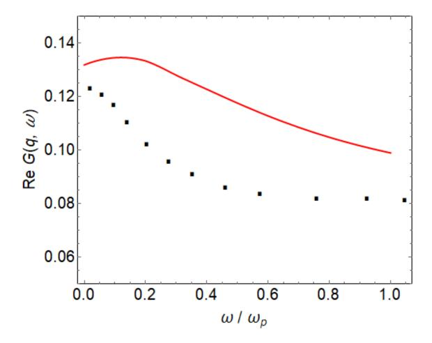
Figure 4.21. Real part of the expression (4.14) for the dynamic local field correction (solid line), compared to the MD results [33] (squares), at q = 1.02 and  $\Gamma = 160$ .
