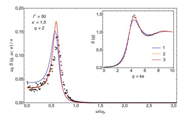
Figure 5.4. Static and dynamic structure factors in YOCP, compared to the MD results (dots) [32]. The static structure factors were calculated using the following schemes: 1 - [30], 2 - [37], 3 - [38,39], 4 - [31].
