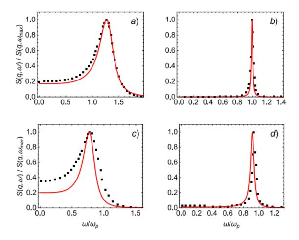
Figure 4.5. The comparison of COCP DSFs, calculated as eq. (4.7) (solid lines) and obtained from MD simulations [33] (squares),
