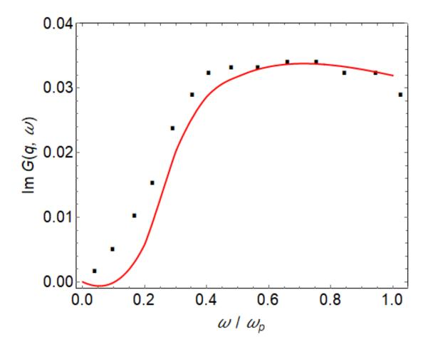
Figure 4.18. Imaginary part of the expression (4.14) for the dynamic local field correction (solid line), compared to the MD results [33] (squares), at q = 1.02 and  $\Gamma = 50$ .
