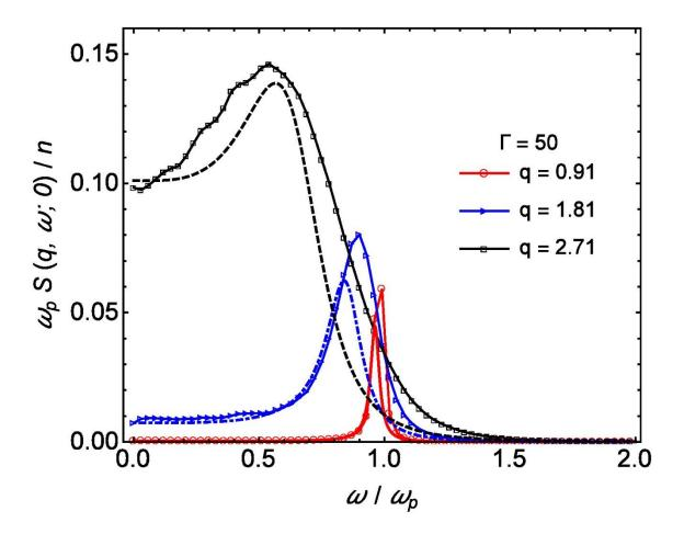
Figure 4.2. The comparison of COCP DSFs, calculated as eq. (4.7) (lines) and obtained from MD simulations [32] (lines with symbols).
