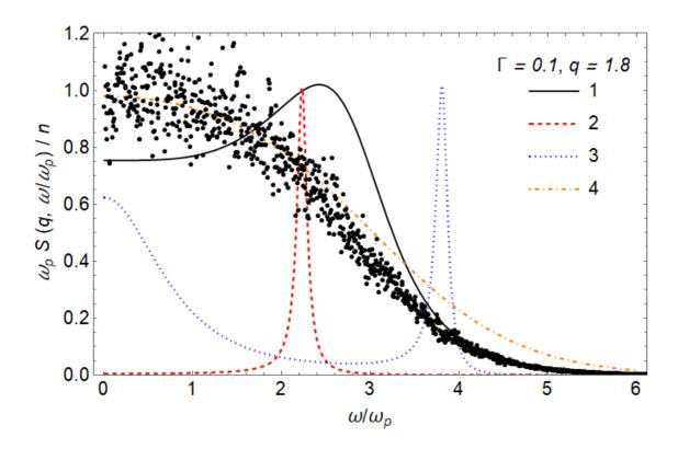
Figure 6.4. Dynamic structure factor fot the COCP presenting the method of moments (MM) data vs. the MD data (dots) [32].
