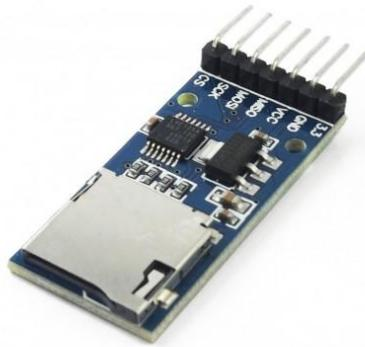
**Figura 9:** Módulo microSD. Fuente: <https://naylampmechatronics.com/modulos/104-modulo-micro-sd-card.html>
