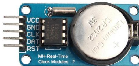
**Figura 3:** Módulo DS1302. Fuente:<https://www.dx.com/p/rtc-ds1302-real-time-clock-module-for-Arduino-avr-arm-pic-smd-2062445#.XQAKWogza70>
