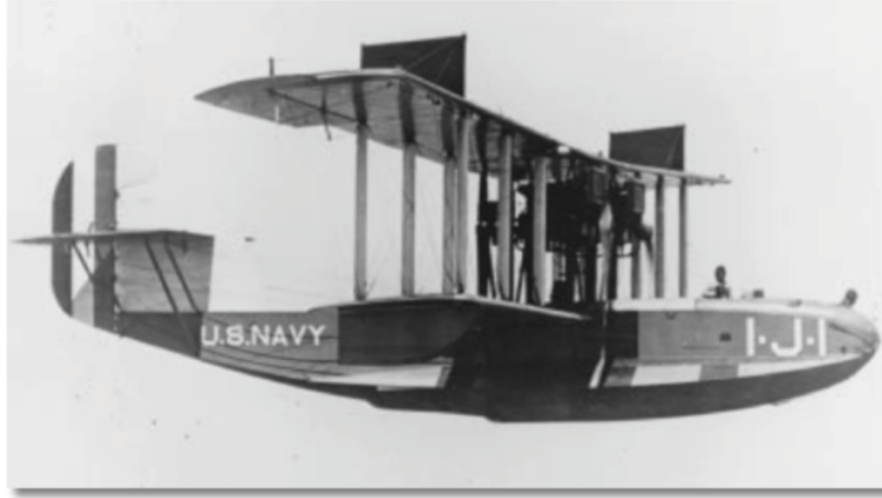
Figure 1.4: On 15 September 1924, radio controlled Curtiss F – 5L flown remotely during all phases of flight, being the first aircraft in history of flight in achieving this. Taken from [8].
