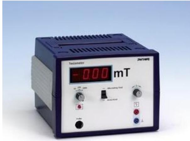
Fig 31. PHYWE TESLÁMETRO, DIGITAL. Fuente: PHYWE
