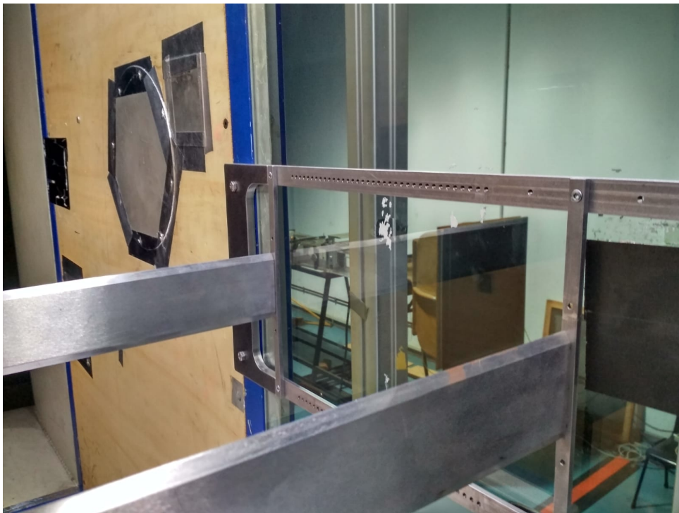
Figure 2.5: Metal strips at the sidewalls of test chamber and steel rod supports mounted for small plate measurements
