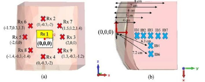
Fig. 3. On-body (a) and in-body (b) antenna locations (top view)
