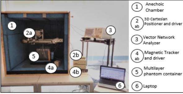
Fig. 1. Laboratory Measurement Setup
