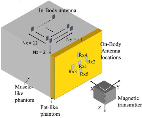
Fig. 2. Measured in-body and on-body positions
