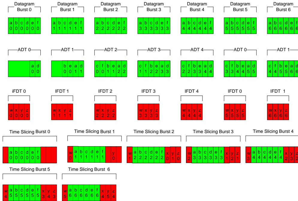
Fig. 8. Example of the RS sliding coding mechanism for C=6, F=4, B=3, D=0 and S=2
