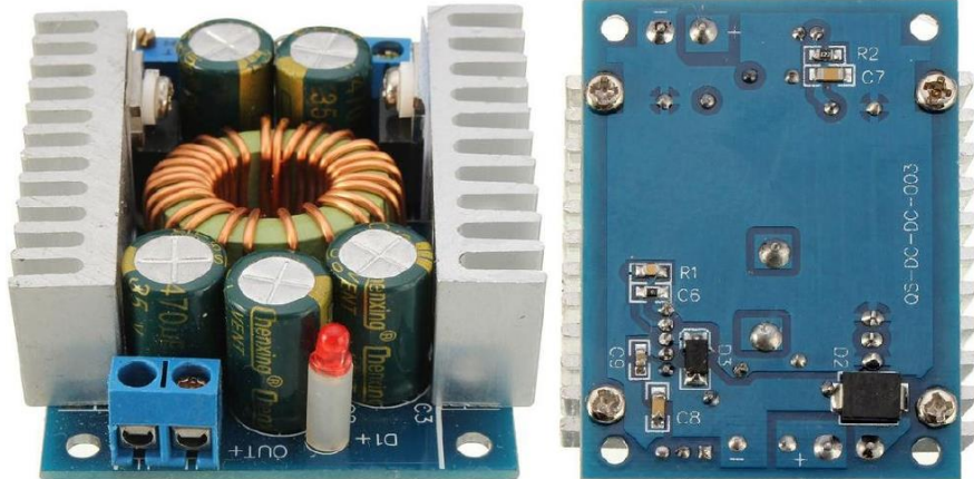
QS-DC-DC-003 DC-DC step down DC-DC converter 1.25-30V, 12A, 100W
