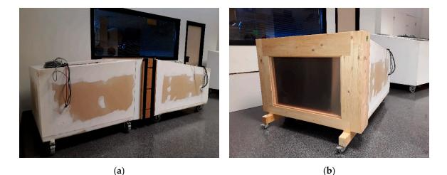
**Figure 1.** Completed reduced sized transmission chamber: (**a**) the two rooms with the sample holder in between; (**b**) view of the sample holder.
