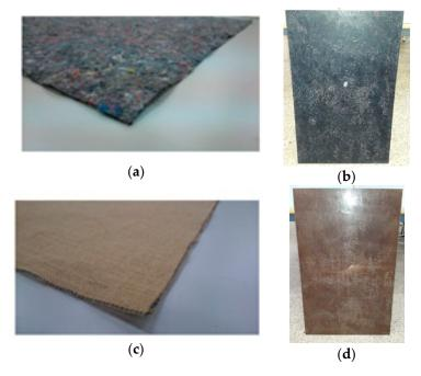
**Figure 4.** (a) Textile waste blanket; (b) textile waste treated with biodegradable resin board; (c) jute fiber blanket; (d) jute fiber treated with biodegradable resin board.
