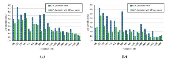
**Figure 3.** Sound pressure level (SPL) deviation for source and receiving rooms: (**a**) source room; (**b**) receiving room.
