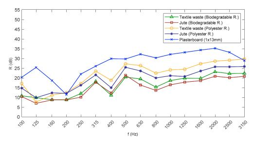
**Figure 6.** Sound reduction index (R (dB)) measured in reduced sized transmission chamber for green composite and plaster boards.
