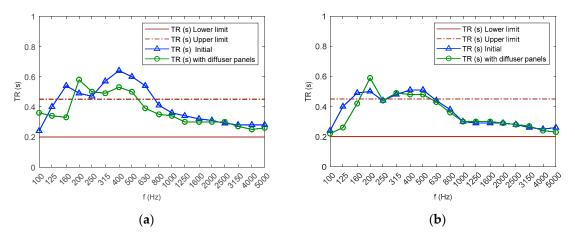
Figure 2. Reverberation time (TR) for source and receiving rooms: (a) source room; (b) receiving room.
