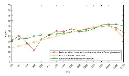
Figure 5. Comparison of the results obtained for a single 13 mm thick plasterboard.
