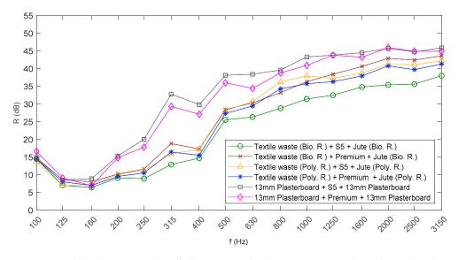
**Figure 9.** Sound reduction index of the proposed solutions measured in the reduced sized transmission chamber.
