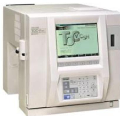
Figura 4.5: Total Organic Carbon Analyzer (TOC)
