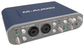
**Figura 18.** Interfaz de audio digital, M-Audio Fast Track Pro
