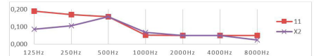
Figure 7. Absorption spectrum of the wooden ceiling panels (after RSM closed curtain-red- after RSM-purple-)
