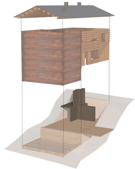
Figure 5. Scheme of black exposed concrete wall inside the house (drawing by the authors).
