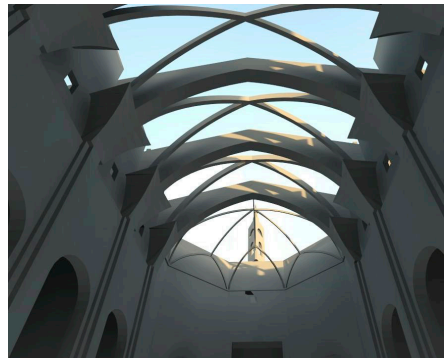
Figure 6. Structural system of Santos Juanes.
