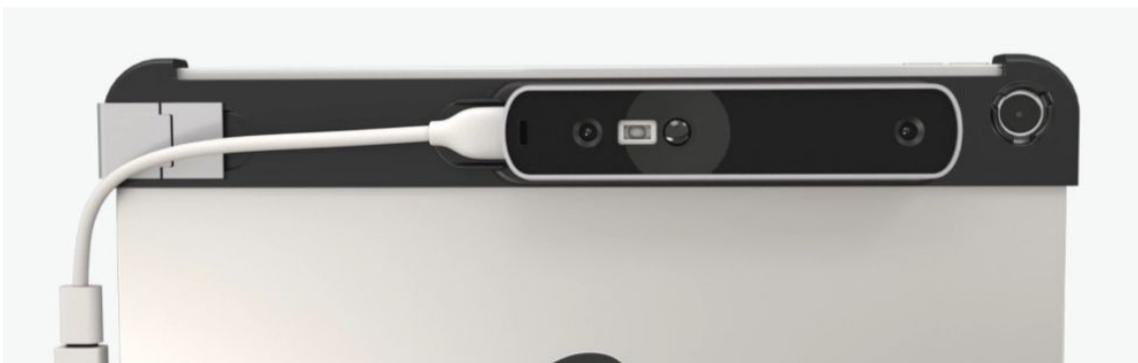
*Figura 2 - Structure Sensor*
