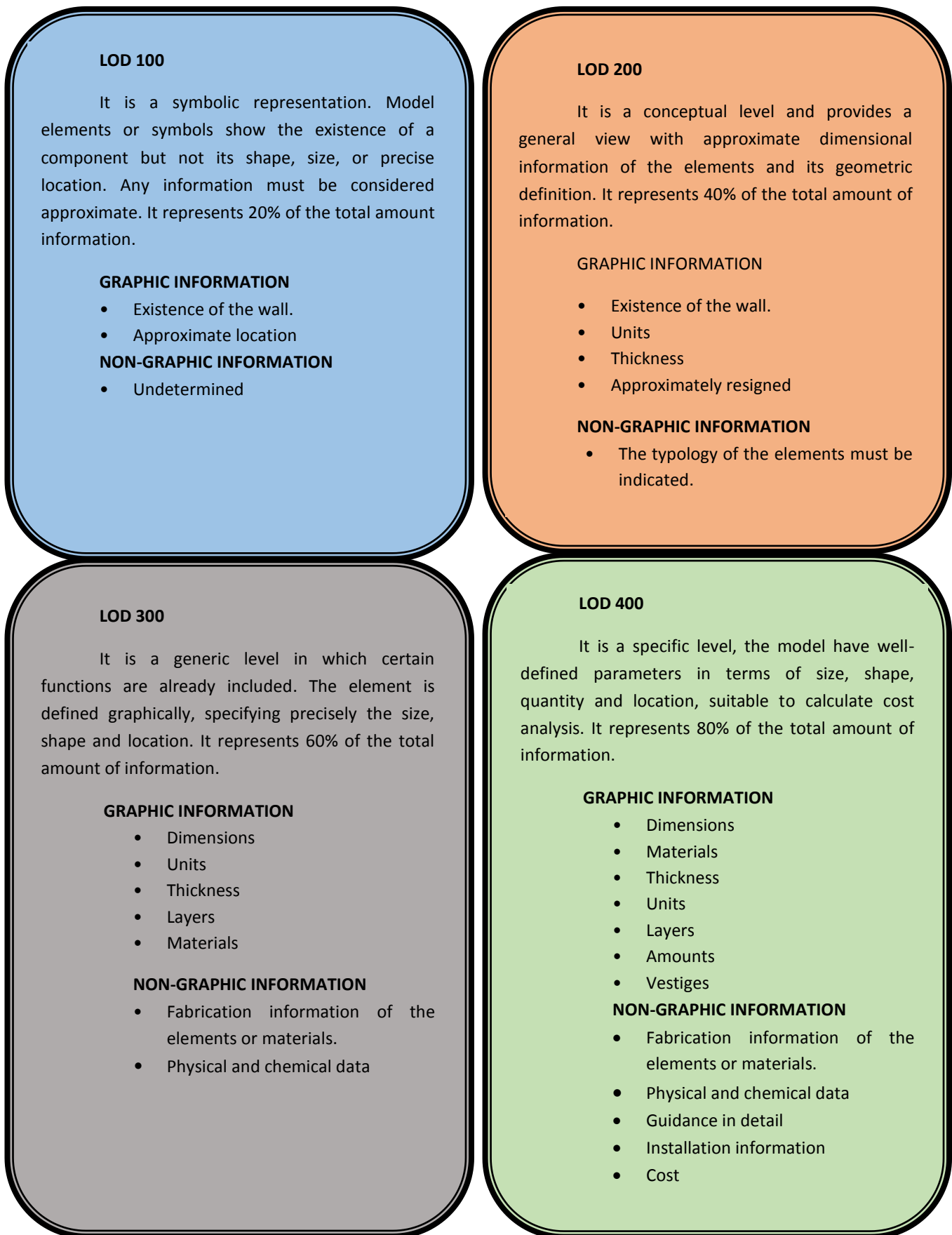
Figure 93. Level of Development for HBIM. Idea suggested by Pr. Jorge García Valdecabres to Mr. Roberto Mogena and corrected by Ms. Isabel Jordán Palomar, 2018.
