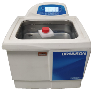
Figure 3.1: Branson ultrasonic cleaner used with a container floating.
