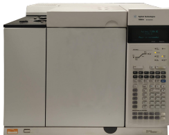
Figure 3.23: Gas chromatograph used. Agilent Technologies model 7890A.
