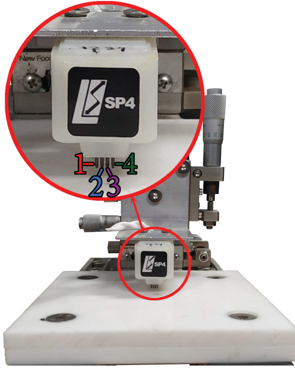
Figure 3.12: Four-point collinear probe used with a zoom in on the probe identifying the four points.
