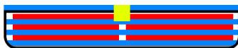
Figure 3.3: Side image explaining the disposition of coated quartz (red), quartz (blue) and tape (yellow) in the crucible (black).
