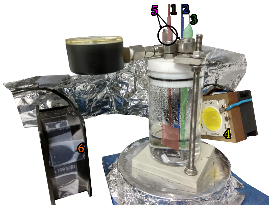
Figure 3.15: Electrochemical cell used. 1: Counter Electrode, 2: Working electrode, 3: Reference electrode, 4: Light source, 5: Gas purging entrance and gas venting and sample taking valve, 6: Cooling fan.
