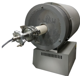
Figure 3.4: Tube furnace used.
