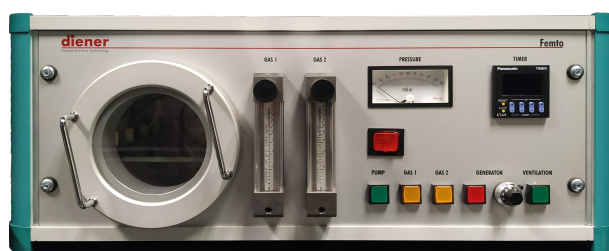
Figure 3.6: Diener Femto plasma cleaner used to treat the ml-G films.
