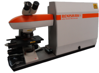
Figure 3.9: Renishaw branded Raman spectrophotometer used.
