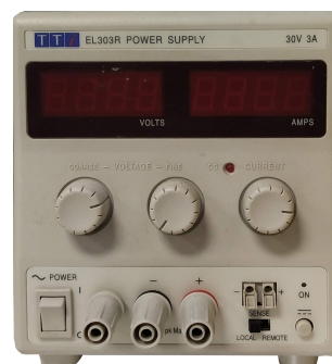
Figure 3.16: DC power supply used. Model EL303R branded by AimTTi.
