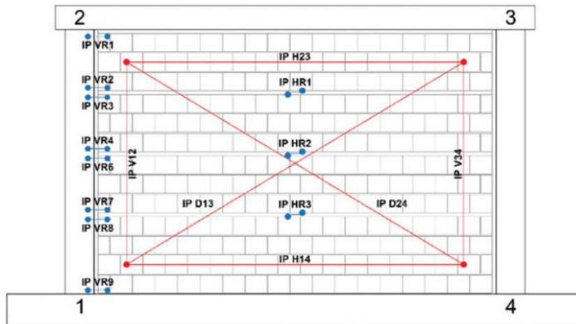
Figure 10. Instrumentation for the in-plane testing (Verlato et al., 2016: p.1362).
