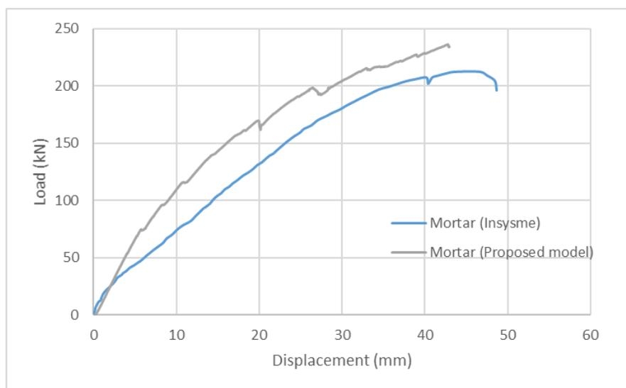
Figure 37. Load-displacement results for mortar models.
