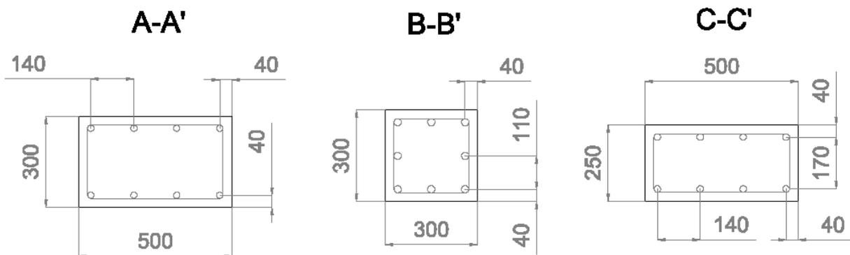
Figure 23. Cross sections of beams and columns. Dimensions in mm.
