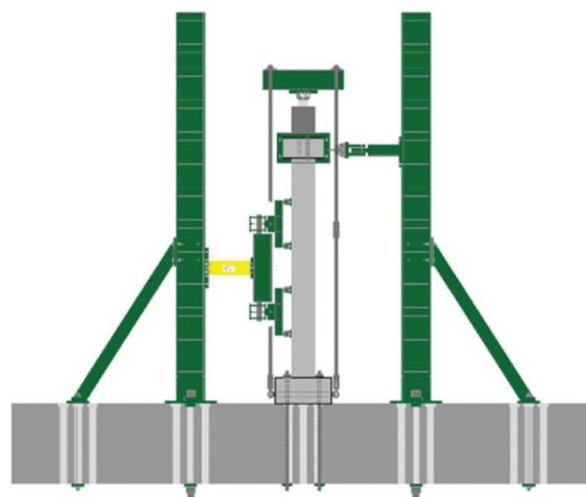
Figure 8. Out-of-plane testing equipment (Verlato et al., 2016: p.1359).
