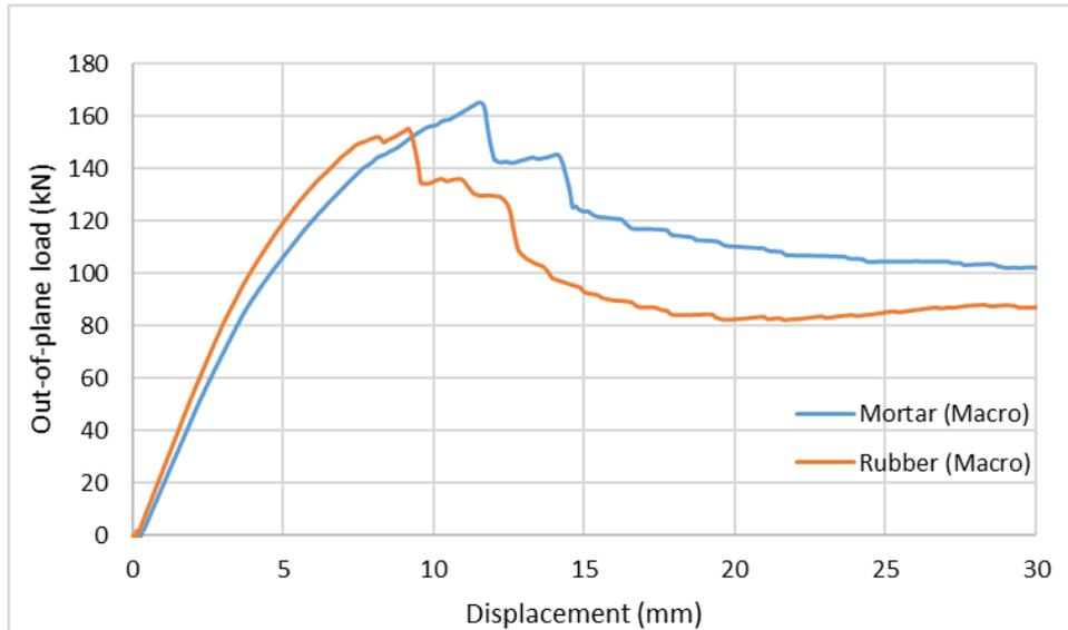
Figure 35. Out-of-plane load-displacement graphs for macroscale models.
