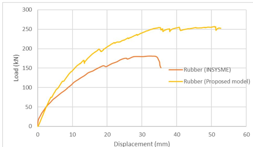
Figure 38. Load-displacement results for rubber models.
