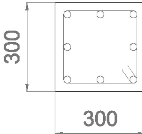
Figure 2. Cross section of columns. Dimensions in mm.
