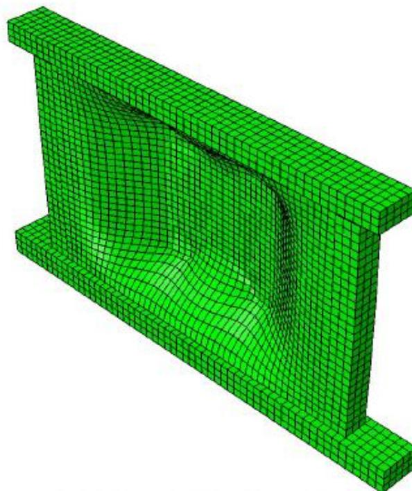
Figure 33. Deformed shape of macroscale model with mortar joints.
