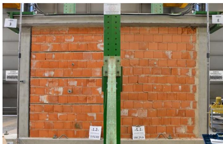
Figure 18. Behaviour of RJ and MJ walls during in plane test at 1.2% drift (INSYSME, 2013).
