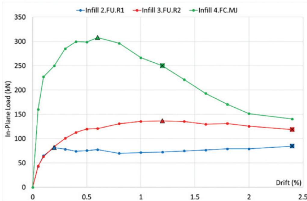
Figure 16. Infill contribution in the in-plane tests (Verlato et al., 2016).
