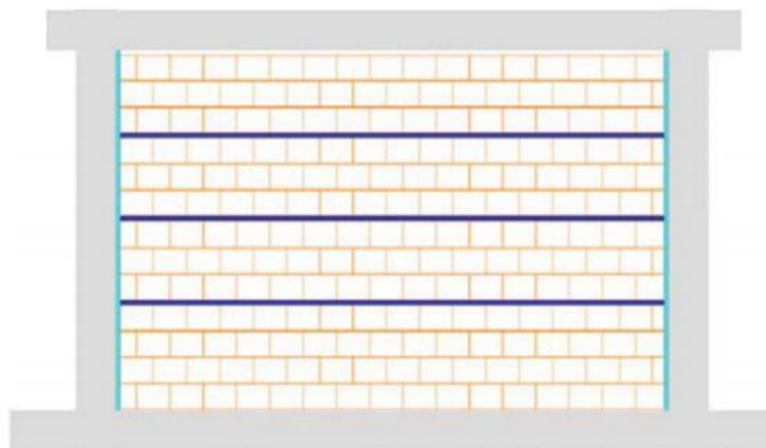
Figure 5. Distribution of rubber joints. Adapted from Calabria et al., (2016: p.1156).
