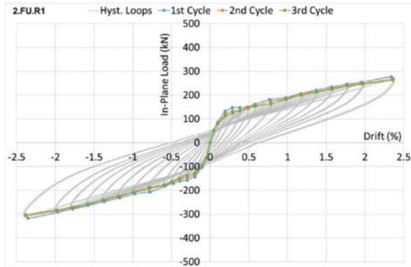
Figure 13. Envelope curves of in-plane test on FU.R1 (Verlato et al., 2016).
