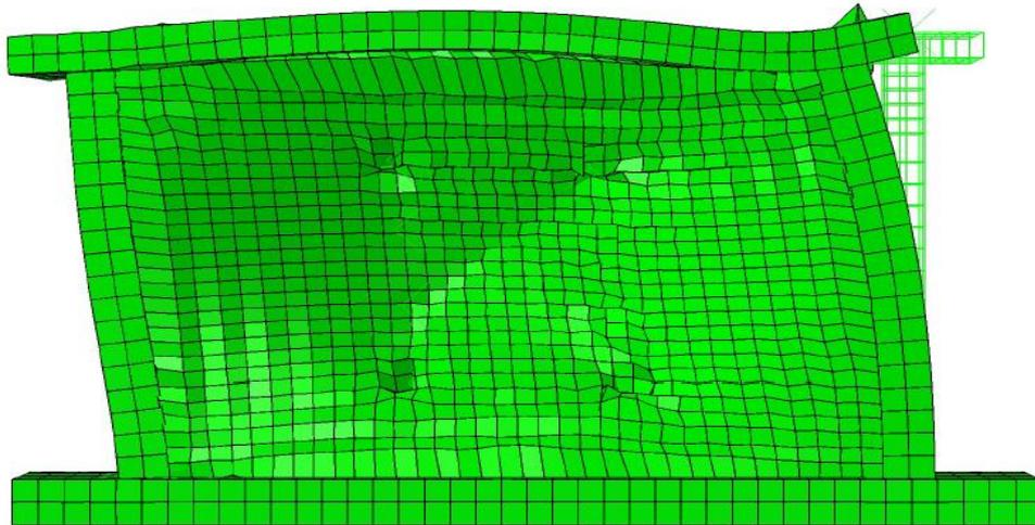
Figure 36. Deformed shape of the mesoscale model with mortar joints.
