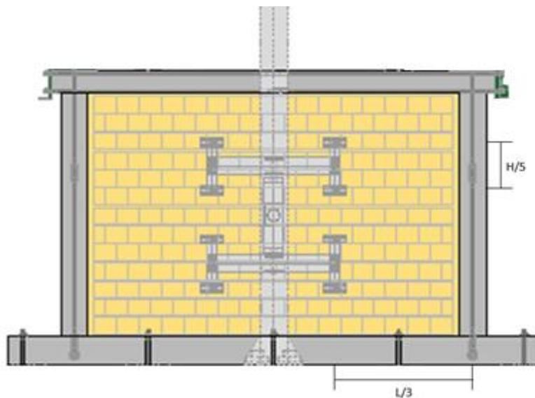
Figure 6. Application of out-of-plane loads. Adapted from Verlato et al., (2016: p.1361).
