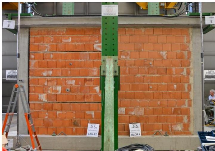
Figure 17. Behaviour of RJ and MJ walls during in plane test at 0.5% drift (INSYSME, 2013).
