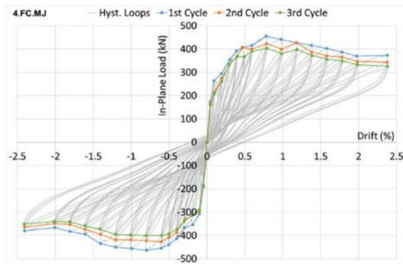
Figure 12. Envelope curves of in-plane test on FC.MJ (Verlato et al., 2016).
