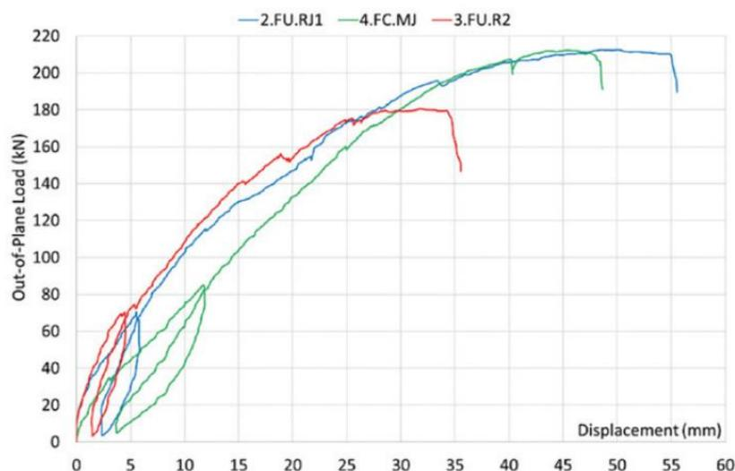
Figure 20. Out-of-plane results of the experimental models (Verlato et al., 2016: p.1365).
