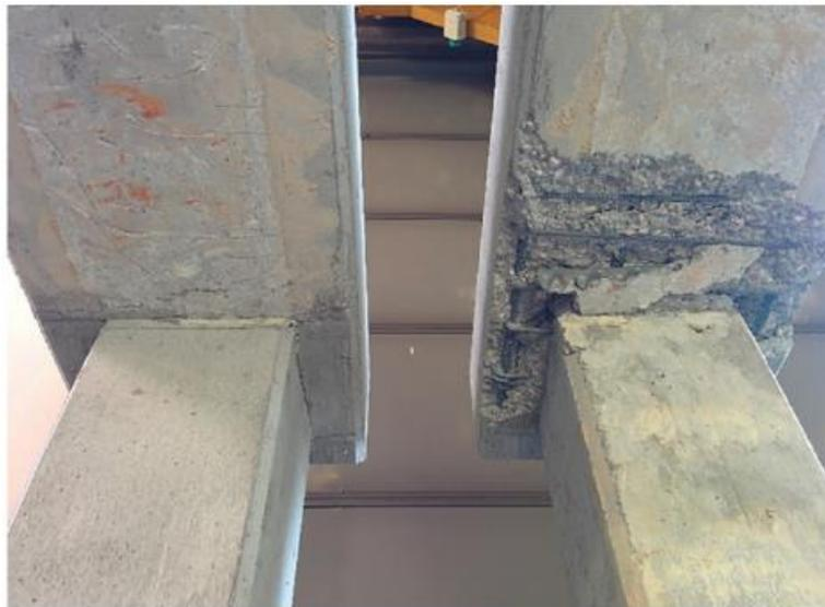
Figure 15. Left to right, FU.R2 and FC.MJ frames after in-plane test (Verlato et al., 2016).
