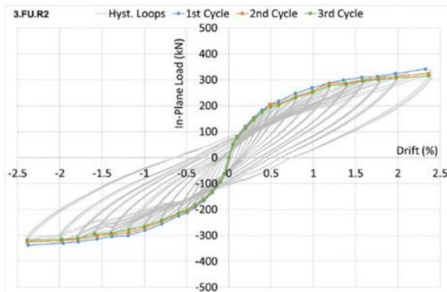
Figure 14. Envelope curves of in-plane test on FU.R2 (Verlato et al., 2016).
