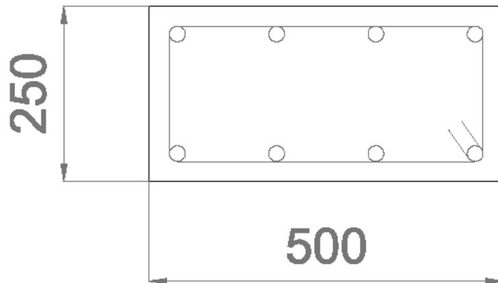
Figure 3. Cross section of top beam. Dimensions in mm.
