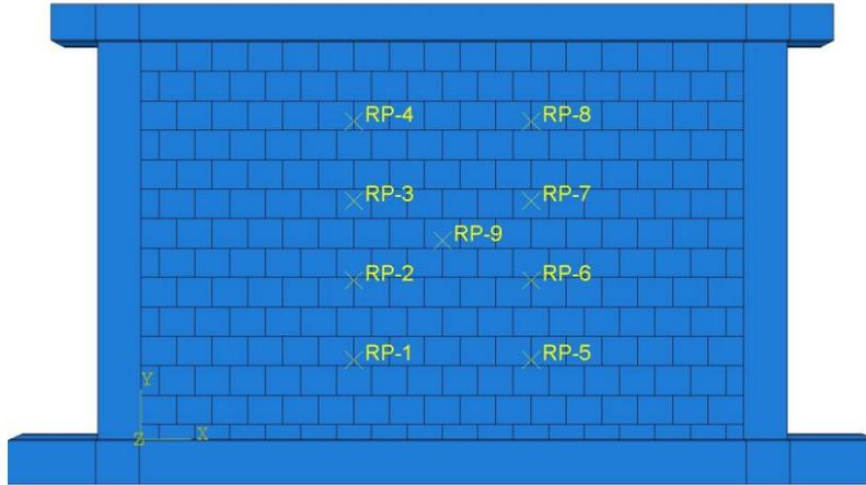
Figure 31. Mesoscale model with mortar joints.
