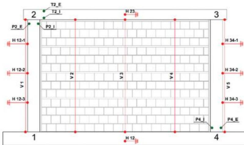
Figure 9. Distribution of the instrumentation in the frame (Verlato et al., 2016: p.1362).
