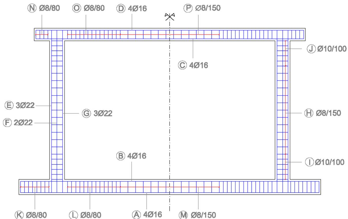
Figure 24. Distribution of the reinforcement in the numerical models.
