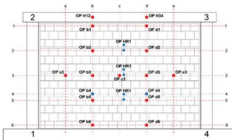
Figure 11. Instrumentation for out-of-plane testing (Verlato et al., 2016: p.1362).
