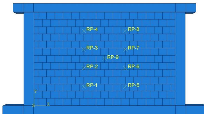
Figure 32. Mesoscale model of wall with rubber joints.
