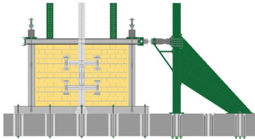
Figure 7. In-plane testing equipment (Verlato et al., 2016: p.1359).
