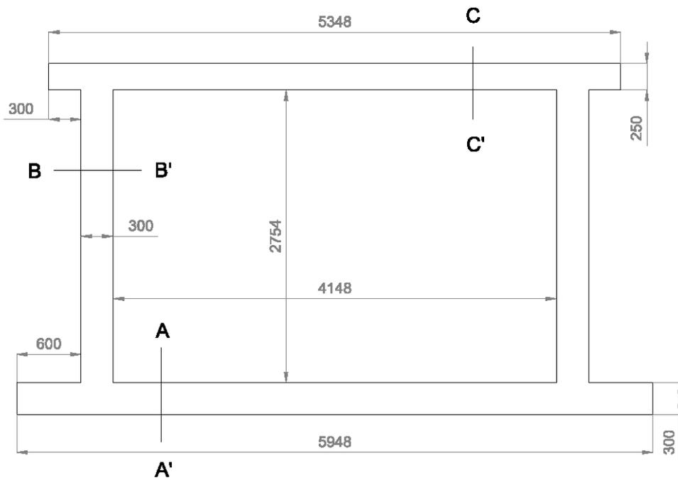
Figure 22. Wall dimensions for the numerical models. Dimensions in mm.
