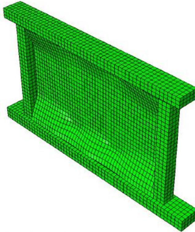
*Figure 34. Deformed shape of the macroscale model with rubber joints.*
