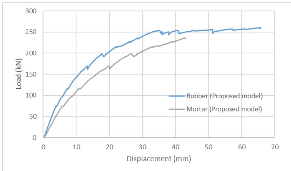
Figure 39. Load-displacement results for mesoscale models.
