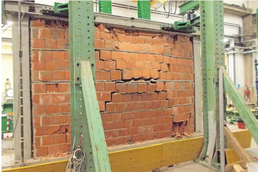
Figure 21. Deformation of the experimental wall with rubber joints (LATERIZIO, n.d.).
