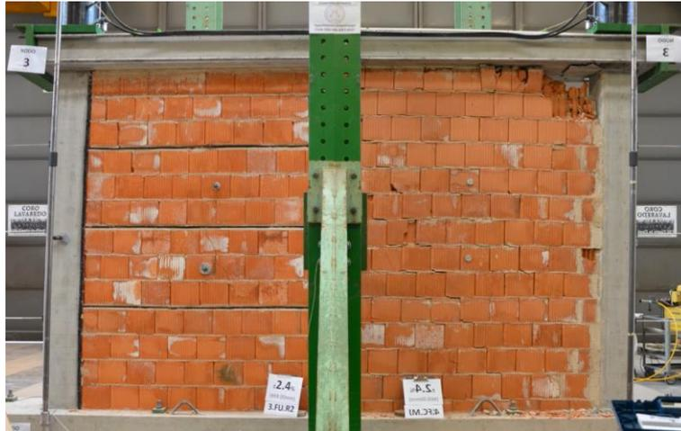
Figure 19. Behaviour of RJ and MJ walls during in plane test at 2.4% drift (INSYSME, 2013).
