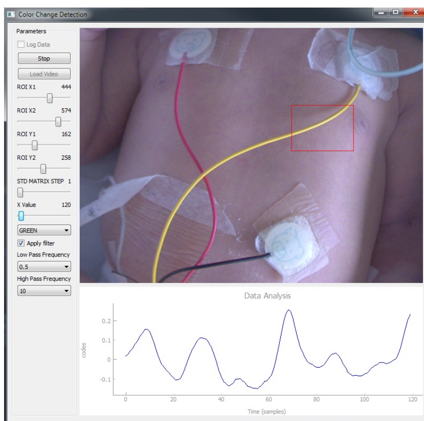
Figure 2.13: Designed application in order to visualize the acquired signal in the ROI while the video is playing and processing.
