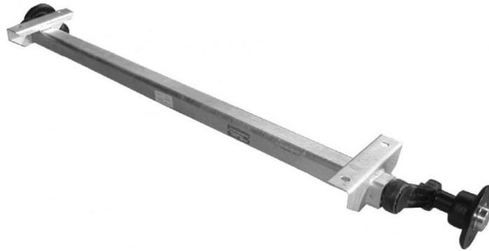
Figura 86: Eje Knott VG7L
